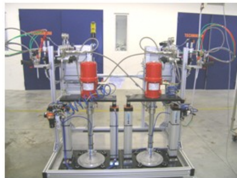
Follower-plates: Transfers material from bucket to Bartec metering pumps
